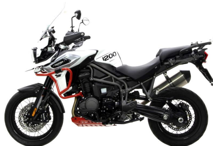
ALUMINUM TRAIL CRASH BAR TRIUMPH TIGER 1200 XCa 2018-2019 TRIUMPH TIGER 1200 XCx 2018-2019 Ref.: 2CP1970048
